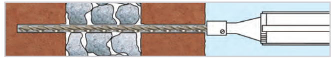
2. Push CemTie fully into grout-filled pinning nozzle of grout gun and insert nozzle to the back of the hole
